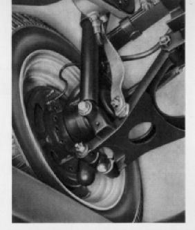
Both the front wheels have been suspended independently at the upper cross leaf spring and the lower steering arms either to the right or to the left sides respectively.
